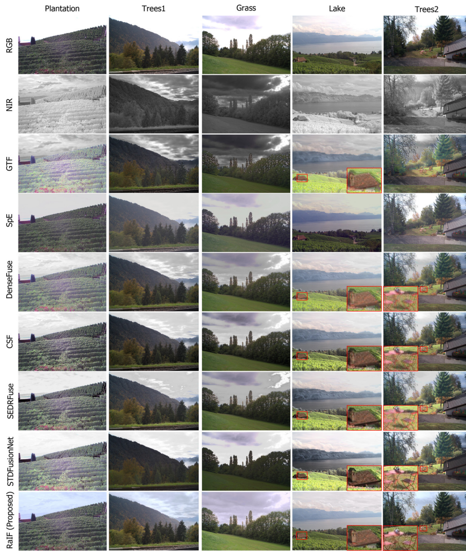
Fig. 11. Image fusion results of 5 scenes in the SKY-OVEREXPOSED group, produced by GTF [13], SpE [14], DenseFuse [8], CSF [17], SEDRFuse [16], STDFusionNet [18], and RaIF. Red boxes highlight the image fusion quality of GTF, DenseFuse, CSF, SEDRFuse, STDFusionNet, and RaIF.
